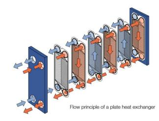
is transferred through the thin plate between the channels, and complete counter current flow is created for highest possible efficiency.No intermixing of the media or leakage to the surroundings will take place as gaskets around the edges of the plates seal the unit. The corrugation of the plates provides a suitable passage between the plates, support of each plate against the adjacent one and a strong turbulence resulting in maximum heat transfer efficiency.
